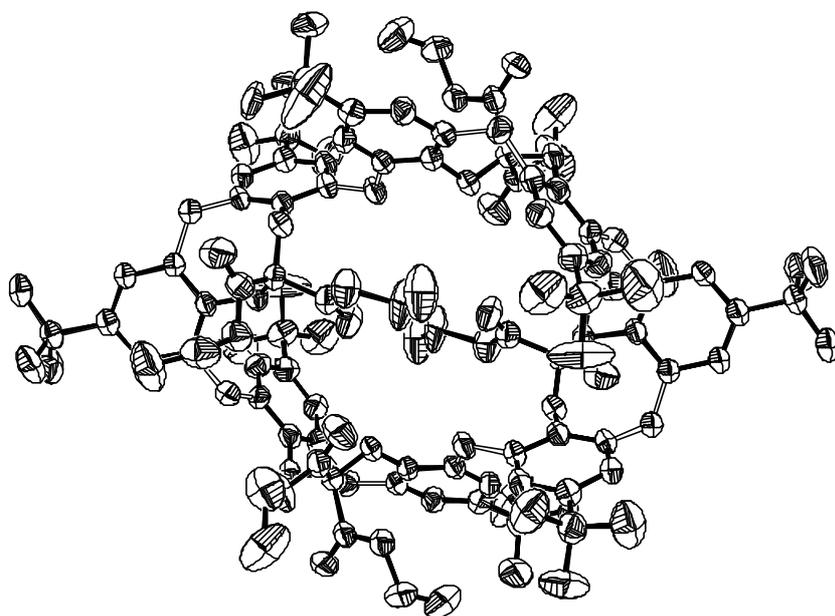
ORTEP drawing for the structure of  $C_{116}H_{144}O_{24}$  with 35% probability ellipsoids
